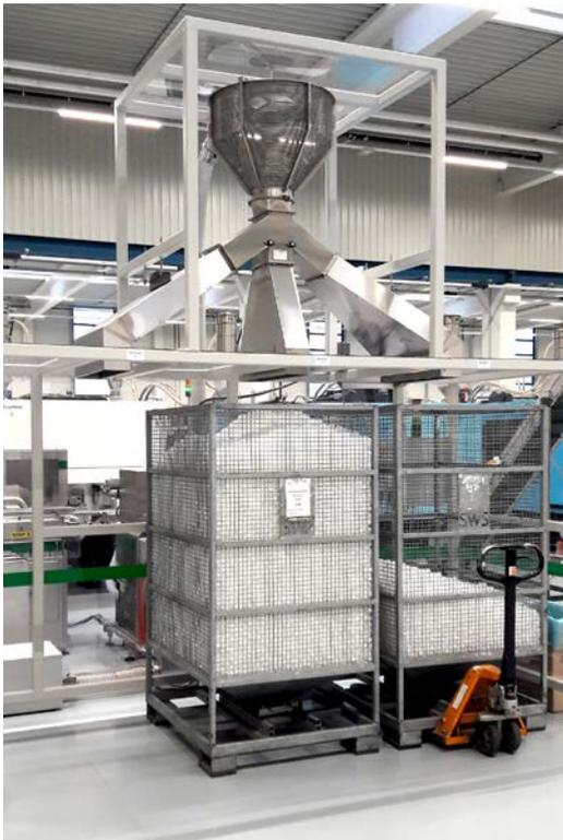
*Opposite of plastic pipes used in conventional conveyor belt system, the trio-technik AirMove system use steel pipes, which are designed for frictionless movement of parts in order to prevent damage on closures during transport.*
