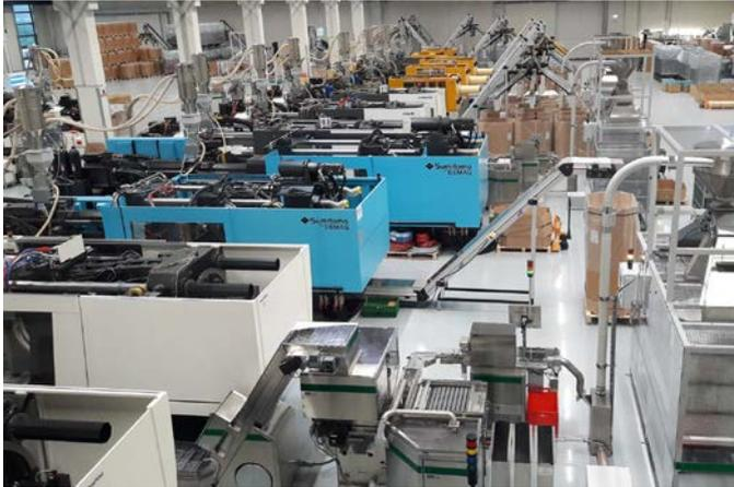
*Thanks to the trio-technik AirMove transport system (on the right on the picture) installed beginning of January 2018, UNITED CAPS only needs about one-third of the space a conveyor belt system would require.*
